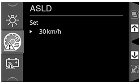
1. ASLD (over speed warning) setting
