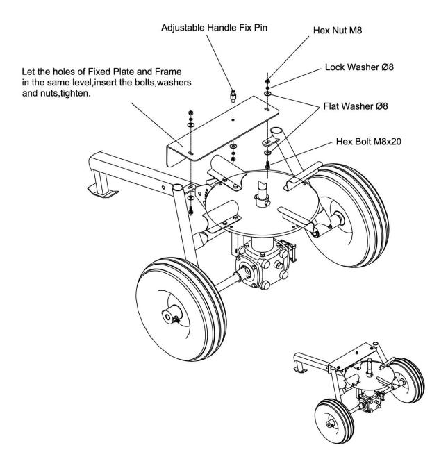
1:Insert the Adjustable Handle into the slot according to the indication in the pic.then put on the bolts,nuts and washers, tighten them to fix the handle and couldn't be moved.
