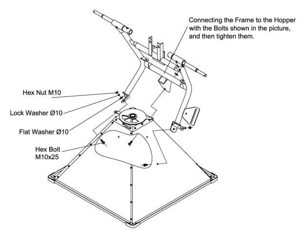
When assembly, please have the hopper side lay, the hopper panel with label should be put in downwards.
