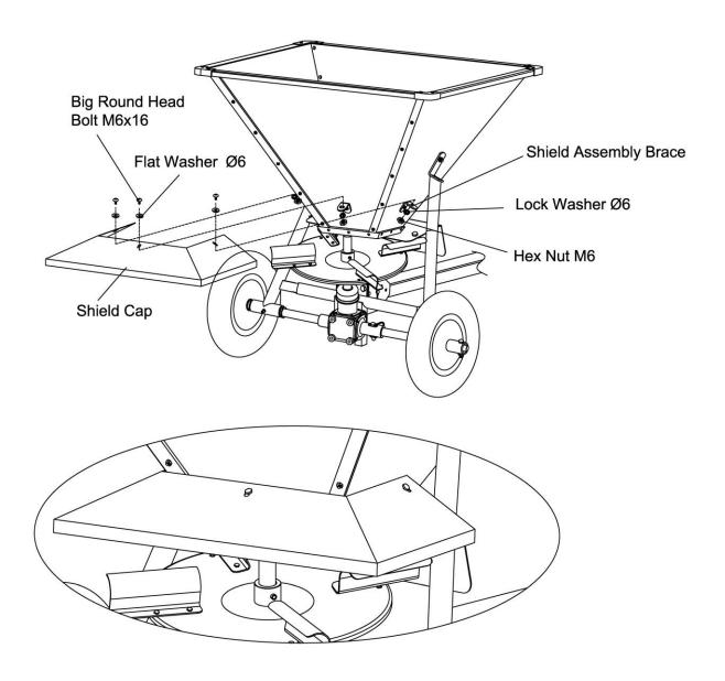
Tighten all bolts as well as the bolts that haven't tighted in the above step.
