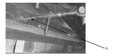
**QUICK OFFSET DRAWBAR** Unlock the nut and screw slide the drawbar to the desired position and release the screw into the securing hole then lock the nut, as shown.
